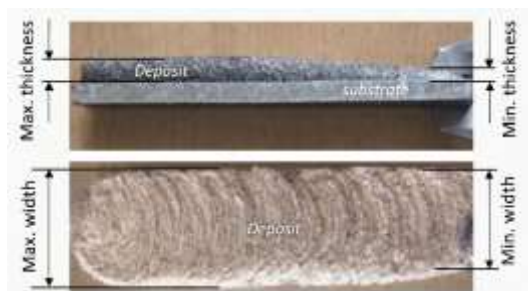
Fig. 3. Width and thickness of the FS-deposited layers
