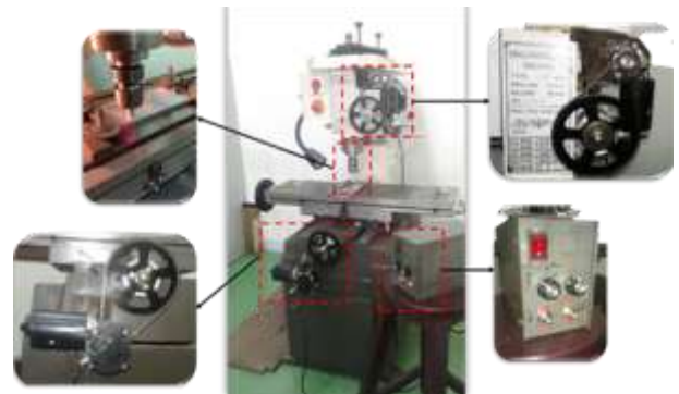
Fig. 1. Modified drilling-milling machine for the friction surfacing process
