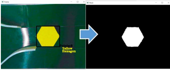
Fig. 7. Masking workpiece yellow color
