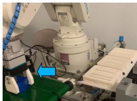
Fig. 19. Robot arm pick workpiece palletizer system based on color
