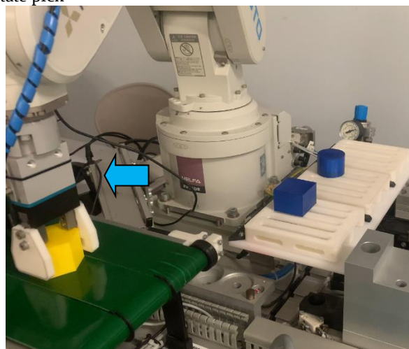
Fig. 15. Robot arm pick workpiece palletizer system based on shape
