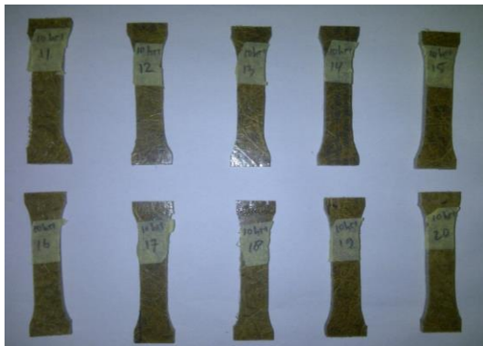
Fig 2. Specimens of compression testing (standar ASTM D695)
