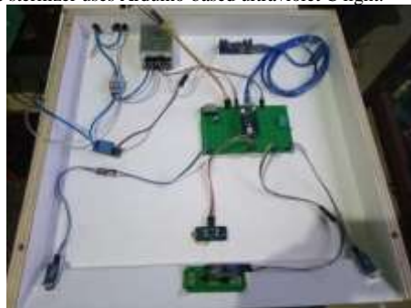
Fig. 3. The electronic circuit of the sterilizer uses Arduino-based ultraviolet C light.
