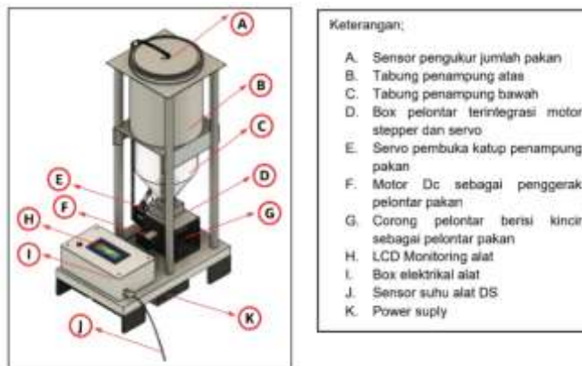
Fig. 1. Isometric view of the feeder design: (A) feed-level sensor, (B) upper hopper, (C) lower hopper, (D) dispersal box with stepper and servo, (E) metering valve servo, (F) DC drive motor, (G) dispersal funnel with impeller, (H) LCD display, (I) electrical enclosure, (J) DS18B20 temperature sensor, (K) power supply.
