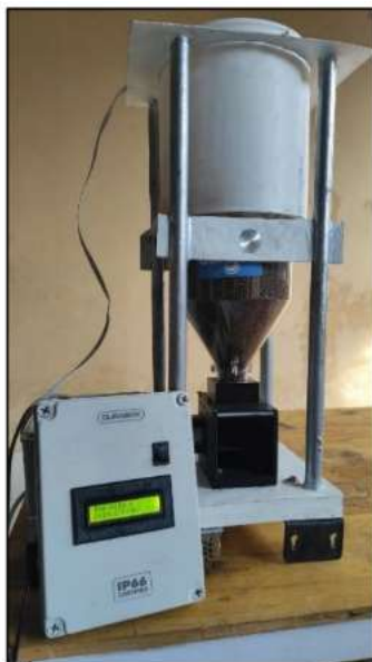
Fig. 2. Realized prototype of the IoT-based automatic fish feeder.
