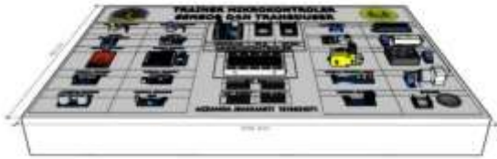
Fig. 2. 3D Design of the Sensor and Transducer Trainer
