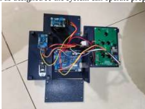
Fig. 5. Results of Installing Cables from Each Component to the Arduino Board
